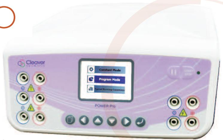
Each power supply has a 2.4" LCD display showing the available options as well as current running conditions. Constant voltage, current and power options are available as well as pre-programmed or customer programmed conditions allowing users to save and repeat their experiments for exceptional reproducibility. The 5 power outlet pairs mean less power supplies are needed for the same number of tanks, saving cost and time when running multiple tanks simultaneously.
